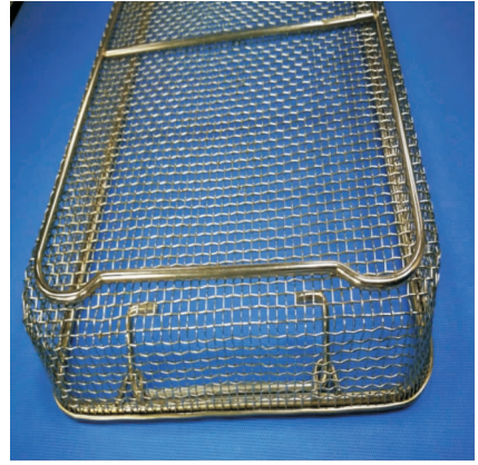
图 2 普通篮筐底部结构 Figure 2 Bottom structure of common basket
